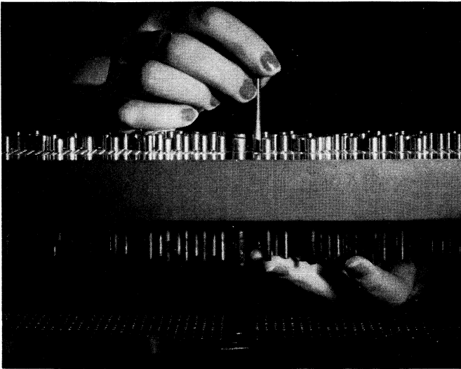
Cutting the Jacquard cards. The weaving process for Wiltons is similar in principle to the operation of a player-piano; the needles in the loom are controlled by a series of pattern cards with holes punched according to the colour appearing on the checked design paper
